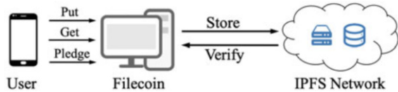
Fig. 3.4 Mechanism and position of Filecoin [11], which is adopted by IPFS and exploits blockchain as its fundamental component
